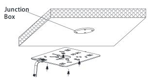
2. Lock the Mounting plate on the embedded Junction box.
