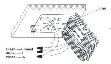
3. Hang the lamp on the ring so as to connect Wire with terminal caps.
