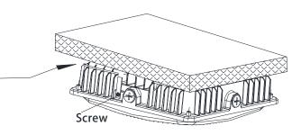
4. Hook up lamp on the mounting plate and Secure the screw, Installation completed.
